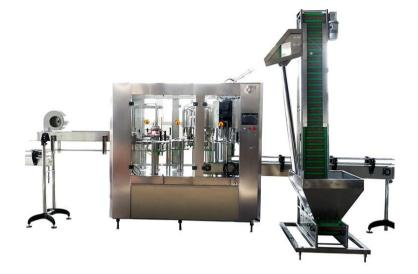
Automatic machine for bottle washing filling and capping, with 18 washing chucks, 18 filling valve and 6 capping heads, production capacity for 500ml mineral water is 4000-6000 bottles per hour. The available bottle sizes for this machine are 300ml – 2000ml.
