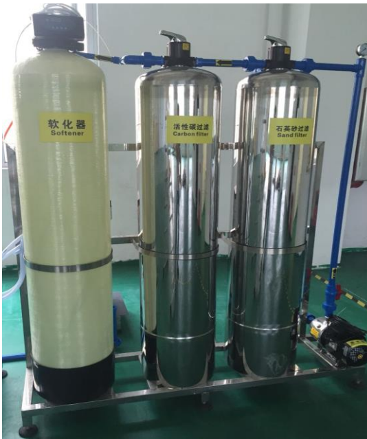
4.6)Prefilter:Sand filter+carbon filter+Softner:
