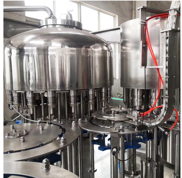
Filling nozzles and Capping heads
