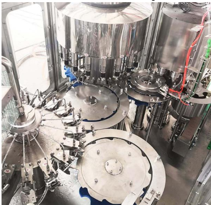
Washing, filling and capping part
