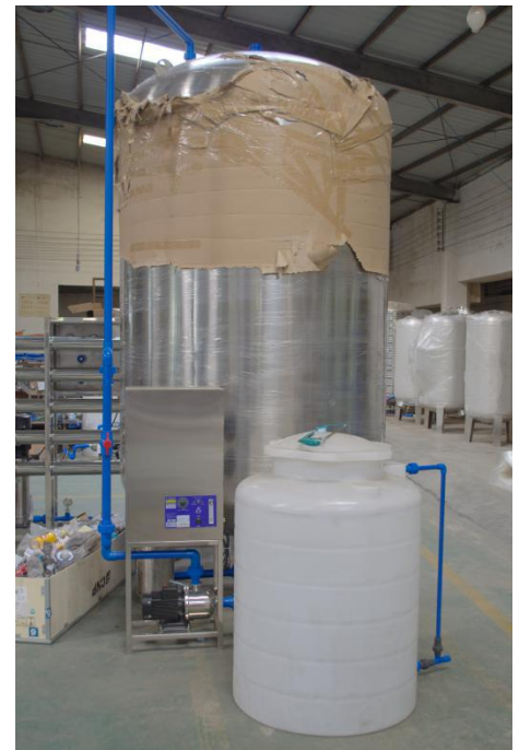
8000L Aspetic Pure Water Tank
