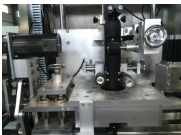
This serial of equipments serves in full auto smart packaging line integrating the functions of bottle delivering bottles and label sleeving. High speed, precise positioning, saving labor and perfect package are the design tenet of this serial of equipments.
